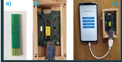
Figure 3 a) Sensor used for analysis. b) Readout circuit. c) Readout circuit connected to sensor and its interfacing with smart phone.
