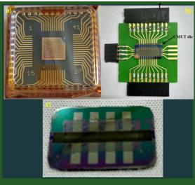
Figure 4. a) Fabricated device of Uncooled IR detector. b) Fabricated SU-8 based CMUT die with wire bonded on to the PCB. c) Fabricated device of Silk-based PMUT.
